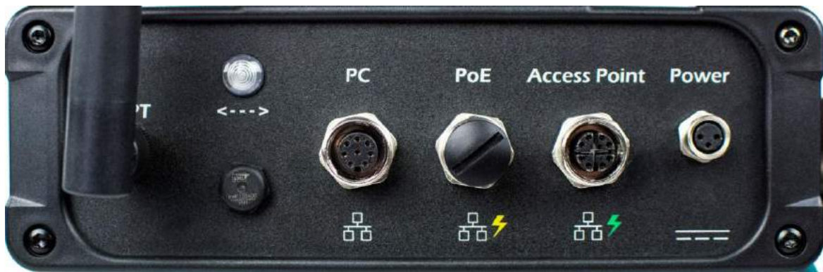
Figure 19: LAN Port Connections
